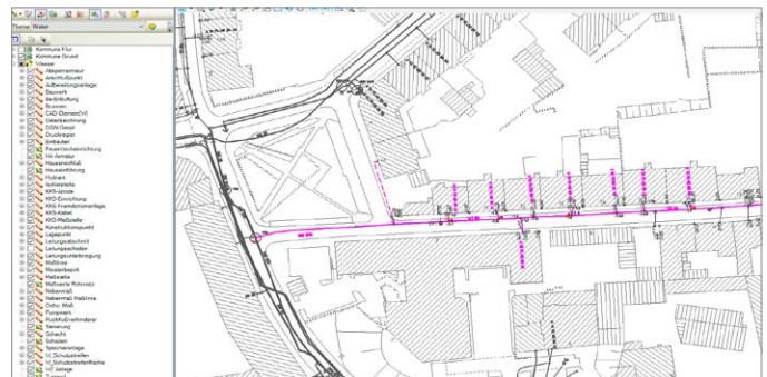
Network trace showing buildings affected by a partial network closure
