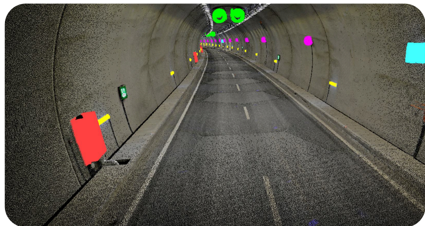
Analyze point clouds and get 3D features for asset inventory – Image courtesy of Yunex
